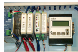
Control Interface with optional User Display, Relay Input, Output and Network Interfaces in pre-wired panel assembly
