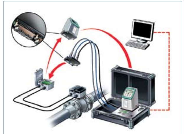
Verificator connection on the SITRANS F M flowmeter
