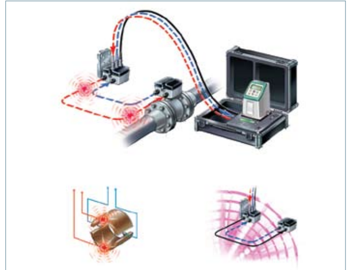
Flowmeter insulation test
