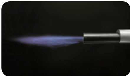
Flame of the ZKIH during natural gas operation in the open air
