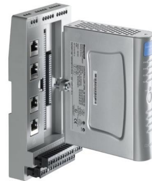
Figure 3. Positive identification on removable terminals
