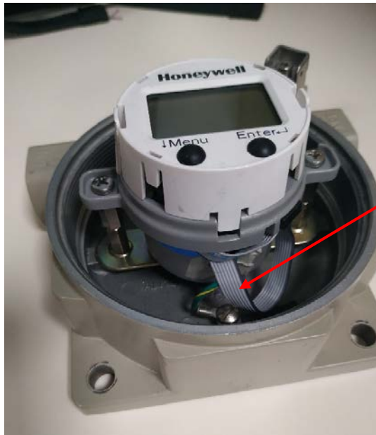
Figure 16: Positioning of Long cable in the IM Housing
