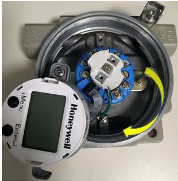
Figure 11: : Position of Standard display for external wiring
