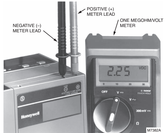
Fig. 8. Measuring voltage flame signal with 7800 Series controls.
