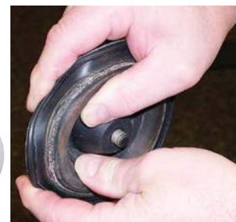
Compare a Steriflow Jorlon™ diaphragm to a competitor's comparable design. The difference, even after a clean steam test, is clear.
