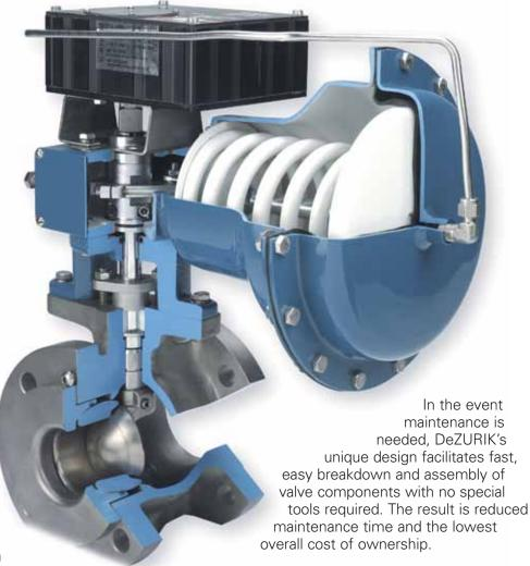
Available in sizes 1–12" (25–300mm), the DeZURIK RCV Rotary Control Valve is available in ANSI 150 and 300 ratings. Body material options include 316 and 317 stainless steel, carbon steel, Hastelloy C or Titanium. Flanged or flangeless designs meet ANSI or ISA face-to-face dimensions.
