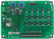
The Series DCT500ADC Low Cost Timer Controller is designed to provide continuous or on-demand cleaning for 10-35 V powered receivers and pulse jet systems. It is available in either 4, 6, or 10 channels, and each unit is the same size, minimizing enclosure space and reducing overall system installation cost. For added safety, the control circuitry including the control inputs are isolated from the line voltage.
