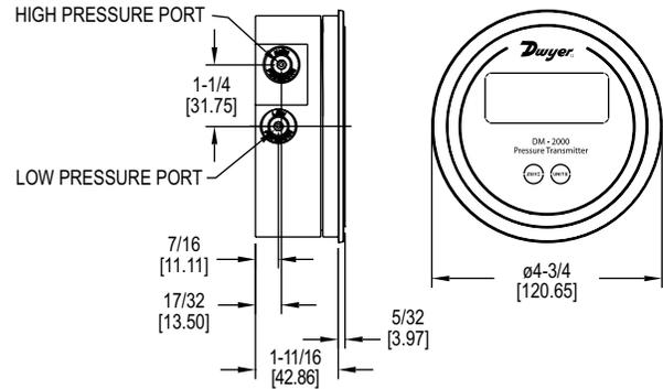
The Dwyer **Series DM-2000 Differential Pressure Transmitters** sense the pressure of air and compatible gases and sends a standard 4-20 mA output signal. The DM-2000 housing is specifically designed to mount in the same diameter cutout as a standard Magnehelic® gage. A wide range of models are available factory calibrated to specific ranges.
