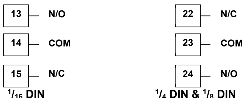
Figure 22. Option Slot 2 - Relay Module
