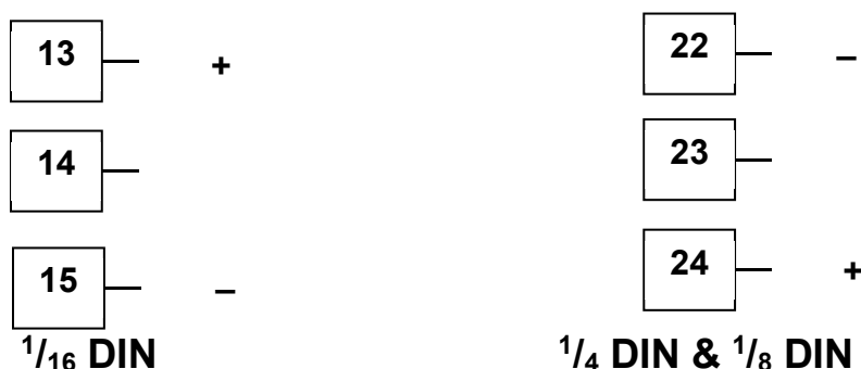
Figure 26. Option Slot 2 - Linear Voltage & mADC module
