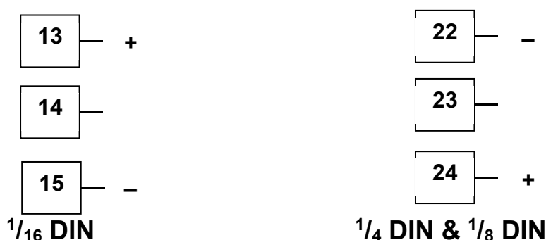
Figure 23. Option Slot 2 - SSR Driver Module
