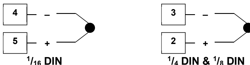
Figure 15. Thermocouple Input Connections
