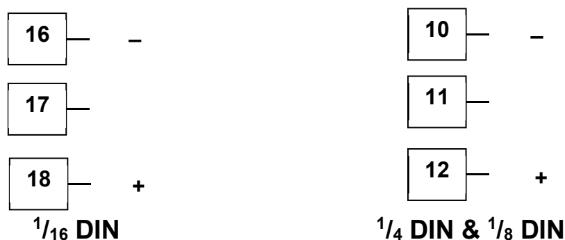
Figure 31. Option Slot 3 - Transmitter Power Supply Module
