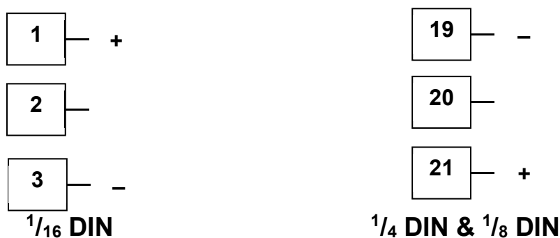
Figure 21. Option Slot 1 - Linear Voltage & mADC Module
