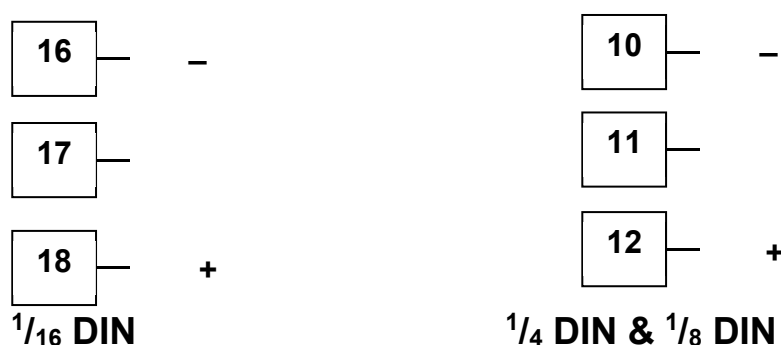
Figure 29. Option Slot 3 - Linear Voltage & mADC module
