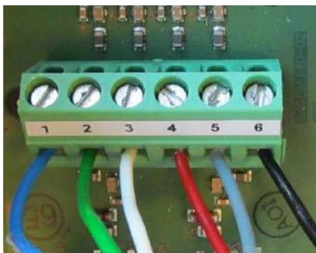
Connect weighing platform to ADU, Option A15
