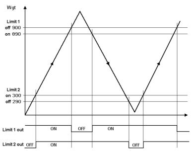
The output signal (Limit 1 out) of limit 1 switches OFF above a weight (Wgt) of 900 g.
