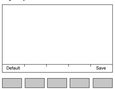
The functions of the five softkeys below the graphic display are indicated in the bottommost text line of the display. Softkey functions shown in gray cannot be selected at the active menu level or with the current access privileges.
