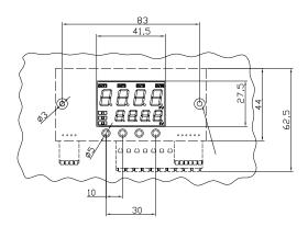
Overall dimensions: 44x91 mm depth 46 mm with 62.5x91mm connectors, depth 46 mm
