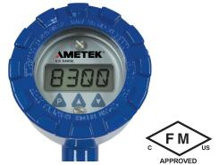
The DT-8300EX is designed for use in process industries, where vibration, inclement weather, and corrosive atmospheres are present. The electronics are enclosed in copper-free, epoxy coated, aluminum housings. The housing is FM explosion proof certified and meets NEMA 4X and IP68 rating standards.
