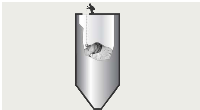
Manual measurement with rope and weight
