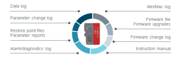
Note that you can even access the manual, either by plugging the microSD card on your laptop or by connecting a USB cable to the LT500.
