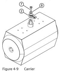
9. Place the positioner and the mount on the actuator carefully. One of the two pins <sup>(12)</sup> of the coupling wheel <sup>(1)</sup> must fit in the carrier <sup>(2)</sup> when you do this.
