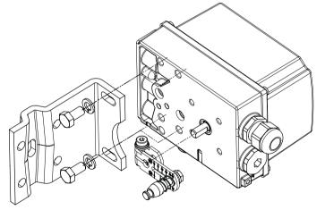
Figure 4-5 Installation with mounting bracket
