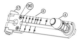
Figure 4-4 Long lever 6DR4004-8L with mounted carrier pin 4 and cylinder head screw 1
