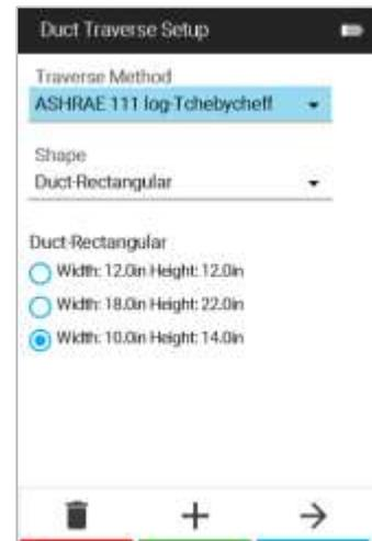
After pressing **+** to add a new duct size, you are brought to the **Flow Setup** page. To change the dimensions, use the arrow keys to navigate between Width and Height then press **←** to begin editing the numbers by using the arrow keys. Press **✓** to save the new duct size.
