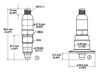
① Thread G½ for hygienic threaded adapter (DIN ISO 228/1) with M12 x 1 plug connection
