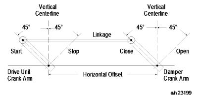
Figure 1 Constant Torque Linkage
