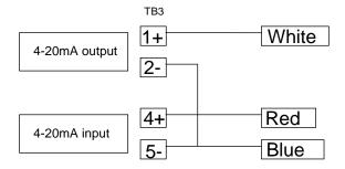
Figure 6 Series 90 connections
