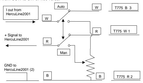
Figure 7 T775 Controller connections
