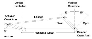
Figure 2 Variable Torque Linkage
