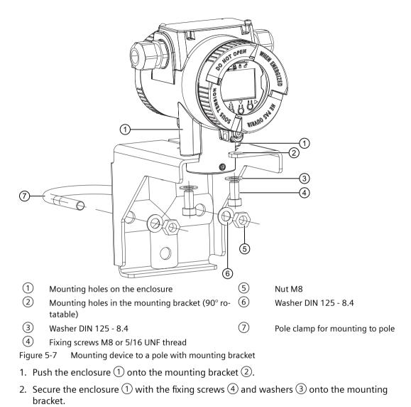
3. Secure the mounting bracket with pole clamp (7), washers (6) and nuts (5) on the pole.
