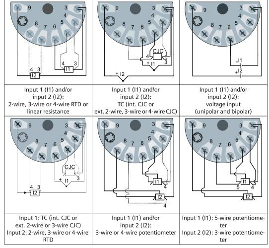
1. Connect the input or inputs to terminals 3 to 9.
