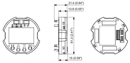
Figure 13-6 Dimension drawings display, dimensions in mm (inch)
