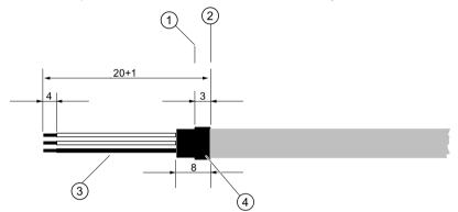
Figure 6-10 Preparing the connecting cable
