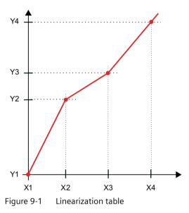
• Set the spline curve (40 breakpoints) (Page 168) Enter the minimum and maximum X-value. The x values are distributed evenly on the x axis according to the desired number of breakpoints. You can freely assign the y values.
