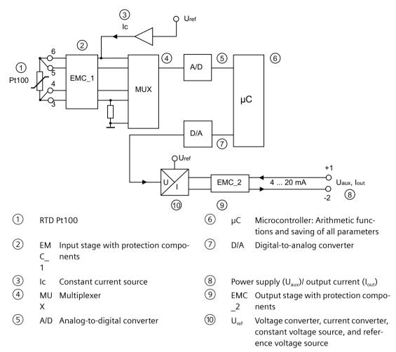
The input and output circuits are each protected against electromagnetic interference through the use of EMC filters.
