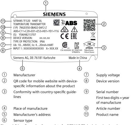
Figure 4-24 Example of nameplate for SITRANS TF dual chamber housing
