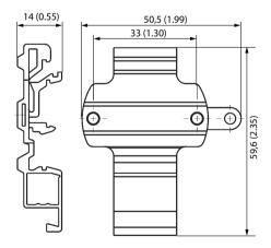
Figure 13-4 Dimension drawings mounting rail adapter (7NG3092-8KA), dimensions in mm (inch)
