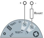
For devices with HART communication, connect a  $\ge 250 \Omega$  resistor.
