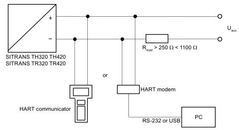
Figure 4-12 HART communication with supply from voltage source
