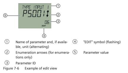
For parameters with an associated unit, the parameter name and unit are displayed as alternating values in 1. Example: Lower range value in °C.
