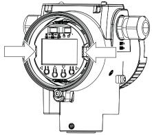
Figure 5-9 Remove the local display
