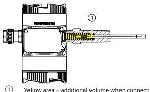
Yellow area = additional volume when connecting a temperature sensor to a SITRANS TF double chamber housing
