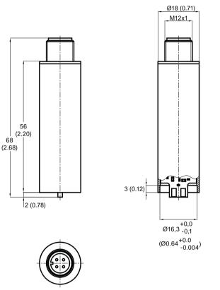
Figure 13-3 SITRANS TH100 Slim dimension drawing, dimensions in mm (inch)
