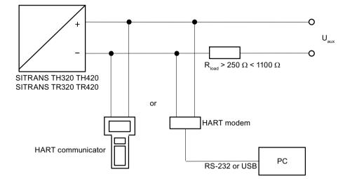
4.3.9.1 HART communication with supply from voltage source
