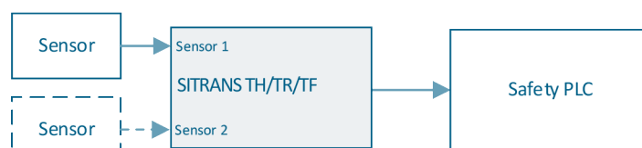
Figure 3 Single transmitter 1oo1 operation (SIL 2)
