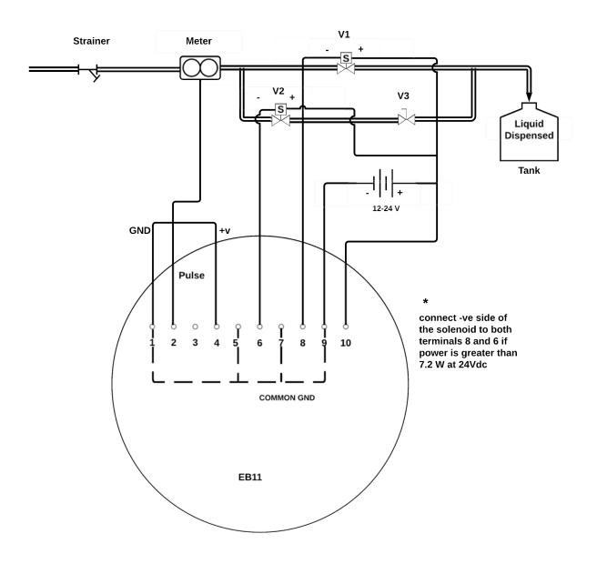
Dual stage system using 24VDC solenoid valves, coil power < 7.2W
