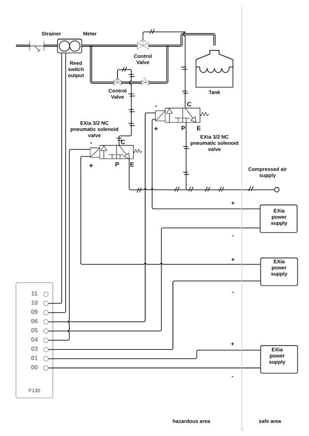
Dual stage system using pneumatic valves (hazardous area)
