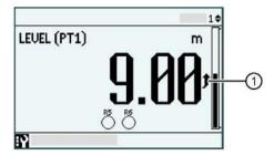
① Filling indicator - appears when view type includes a vertical bar graph and level is increasing faster than the fill rate indicator limit.
