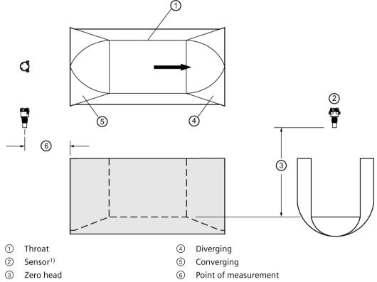
$^{1)}$  The sensor must be above the maximum head by at least the blanking value (Near range (2.1.6.9) (Page 198)).
