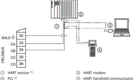
Typical PLC configuration with Passive HART connection
