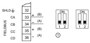
① Termination for Profibus DP (dip switches on Profibus DP card only, normally set in OFF position as shown here)
