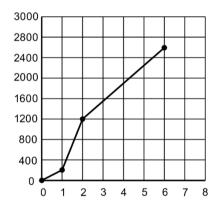
This volume calculation creates a piece-wise linear approximation of the level/volume curve, providing best results if the curve has sharp angles joining relatively linear sections.
