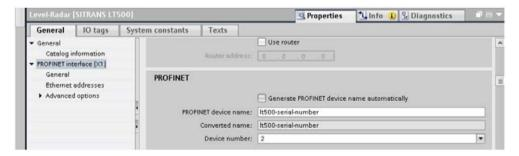
Ensure that the device name matches the device name set in your PROFINET I/O controller or SITRANS LT500 will not establish communication with the I/O controller.
