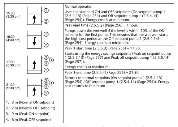
In general, cascade the timing of the pump downs so that the wells farthest from the treatment facility begin first and the entire system pushes material through during the low cost period.
