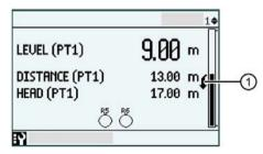
① Emptying indicator - appears when view type includes a vertical bar graph and level is decreasing faster than the empty rate indicator limit.
