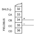
For **Active** HART connection (using LT500 integral power supply), connect terminals 33 and 34.
