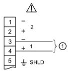
To sensor (measurement point 1) Note that for SITRANS LR110, or SITRANS LR120 connection: positive = black wire negative = white wire
