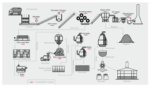
Each of the presses relies on at least 10 switches. Shredders, boilers, cookers, washers and other equipment also use the devices. The conditions are rugged. Canes are wet and muddy. Mills are set in locales where humidity and temperatures run high. Vibration and shock are intense in the machines that perform the processes.
