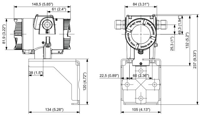
Figure 13-7 SITRANS TF Dual chamber housing dimensional drawings, dimensions in mm (inch)
