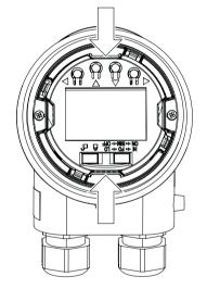
4. Disconnect the cable from the local display.
