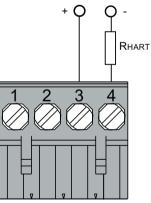
For devices with HART communication, connect a  $\ge$  250  $\Omega$  resistor.
