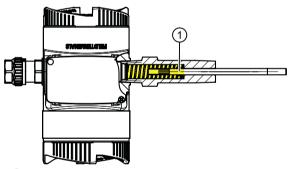
(1) Yellow area = additional volume when connecting a temperature sensor to a SITRANS TF double chamber housing
