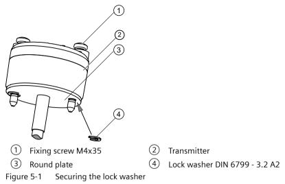
3. Secure the transmitter with the fixing screws in the connection head base.
