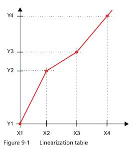
• Set the spline curve (40 breakpoints) (Page 164) Enter the minimum and maximum X-value. The x values are distributed evenly on the x axis according to the desired number of breakpoints. You can freely assign the y values.
