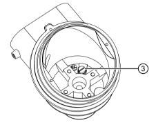
The screw of the ground terminal is electrically connected to the external protective conductor connection.
