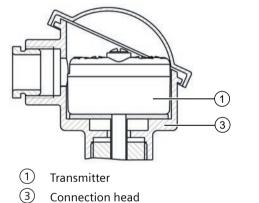
Figure 5-2 Securing the transmitter in the connection head base
