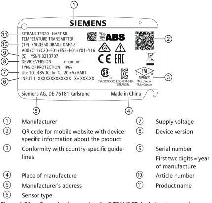
Figure 4-21 Example of nameplate for SITRANS TF dual chamber housing
