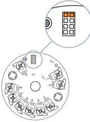
Figure 9-3 SITRANS TH: Enable write protection using the jumper
