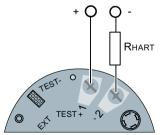
For devices with HART communication, connect a  $\ge 250 \Omega$  resistor.
