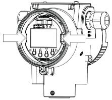
Figure 5-9 Remove the local display
