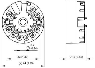
Figure 13-1 SITRANS TH320/TH420 dimension drawings, dimensions in mm (inch)
