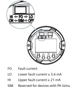
SIM Reserved for devices with PA (simulation mode) Figure 9-7 Set the upper fault current using switch
