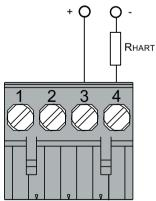
For devices with HART communication, connect a  $\ge$  250  $\Omega$  resistor.
