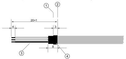
Figure 6-10 Preparing the connecting cable
