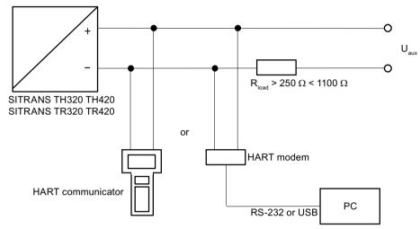
Figure 4-9 HART communication with supply from voltage source
