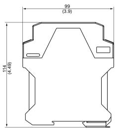
Figure 13-4 SITRANS TR320/TR420 dimension drawings, dimensions in mm (inch)
