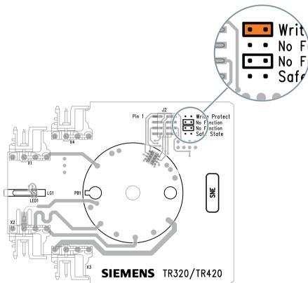
Figure 9-5 SITRANS TH: Enable write protection using the jumper
