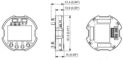
Figure 13-5 Dimension drawings display, dimensions in mm (inch)
