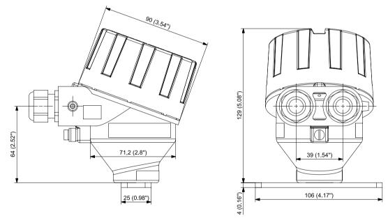
Figure 13-6 SITRANS TF Single chamber housing dimensional drawings, dimensions in mm (inch)
