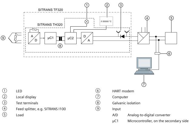
Figure 4-22 Function chart for SITRANS TF with SITRANS TH320
