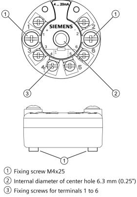
1 (+) Output terminals: Power supply  $U_{aux}$  , output current  $I_{out}$  and 2 (-)
