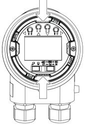
Figure 5-6 Remove the display
