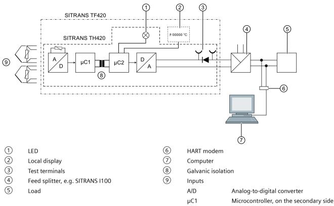
Figure 4-23 Function chart for SITRANS TF with SITRANS TH420
