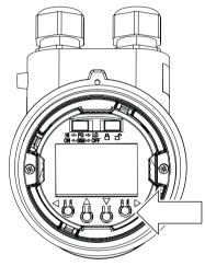
Figure 7-1 Single chamber housing with open cover
