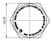
Sealing plug Ex d, M20 x 1.5, dimensions in mm
