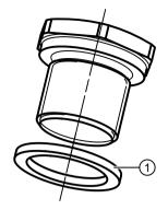
(1) Sealing ring: Use for dust protection "Ex t" type of protection.
