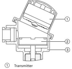
2 Ceramic base of the measuring element
