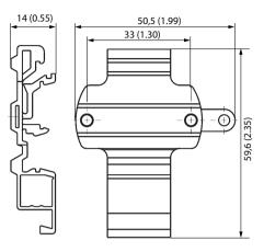
Figure 13-3 Dimension drawings mounting rail adapter (7NG3092-8KA), dimensions in mm (inch)
