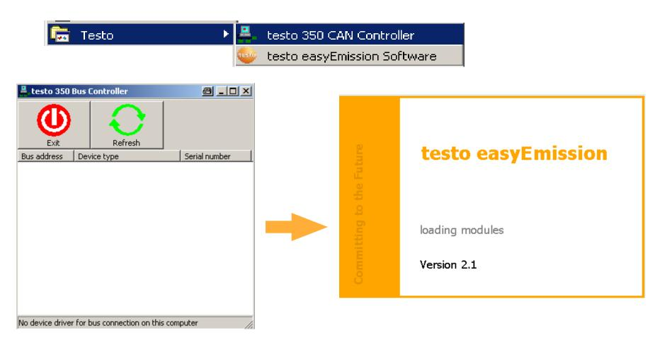
Start first the program testo 350 CAN Controller (connection between CANCase and Computer) and then easyEmission
