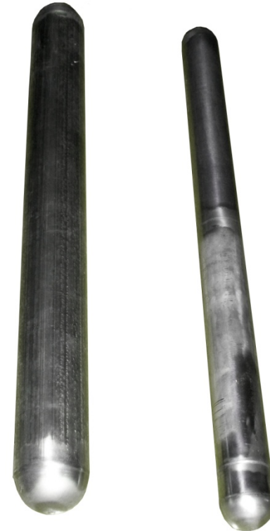
Lower SG Floats, Titanium and Hastelloy
