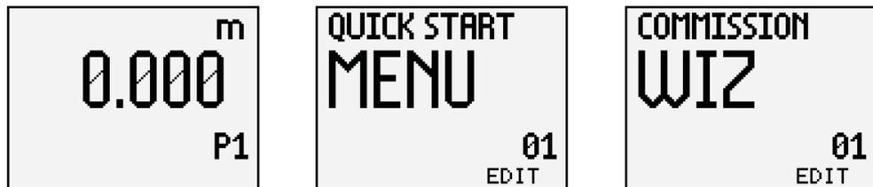
2. Press the " → " button again to start the " Quick Commissioning Wizard" (COMMISSION). In the wizard, it is not necessary to press the " ↓ " button to navigate to the next step. In each step you will be taken directly to the edit view.
