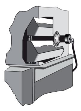
For elevators with ferrous walls, cut 88 to 95 mm (3.5 to 3.75 inch) hole in the elevator wall. Any position from A to C may be used to maintain gap
