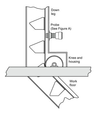
For chain and sprocket drive elevators, place the probe so that the gap between the bucket and the probe does not exceed 102 mm (4 inch). To prevent damage to the probe from eccentric bucket motion, ensure that the gap is not less than 12.5 mm (0.5 inch) in the worst condition
