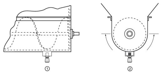
① The probe should be located at the idler end (usually feed end)
