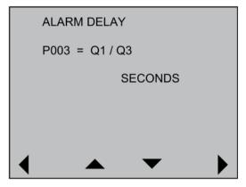
When value = > 0 then output relays are held maintained (Hi) for the set time period to allow system to achieve process speed.
