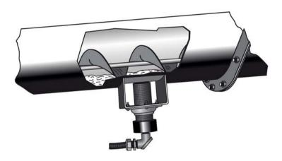
B.9 End Bearing on Screw Conveyor
