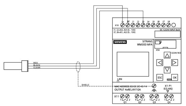
Wire can be run in conduit. Connection to probe terminals can be made under probe cap.
