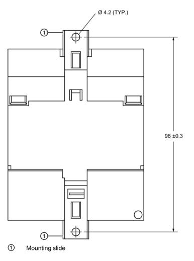
For wall mounting slide the tabs out and mount to the wall/post with M4 screws.
