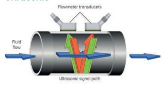
With transit time flow measurement, two transducers serve as both ultrasonic signal generators and receivers. When mounted on a pipe, they are in acoustic communication with each other, meaning the second transducer can receive ultrasonic signals transmitted by the first transducer and vice versa.
