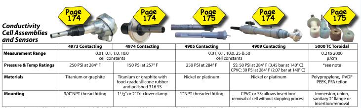
\* Polypropylene: 100 PSI at 212° F (6.9 bar at 100° C) PVDF: 100 PSI at 248° F (6.9 bar at 120° C) PEEK: 200 PSI at 302° F (13.8 bar at 150° C) PFA Teflon: 200 PSI at 302° F (13.8 bar at 150° C)
