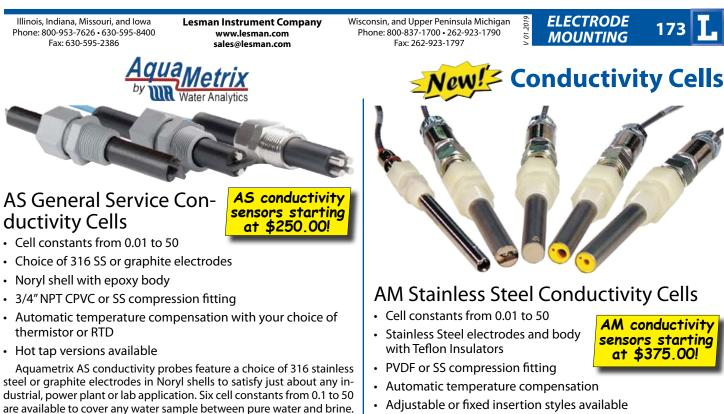
A compression fitting allows for adjustable insertion length in 3/4"NPT piping or in the side of a tank. Reverse the direction of the compression fitting for submersion mounting. A ball valve ("hot-tap") types permit removal of the cell from process piping or from tanks without shutting down the system. All cell types are designed with a safety stop shoulder on the cell.
