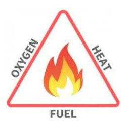
• In order for combustion to occur, we not only need all three of these elements, but we need the proper **ratio** of oxygen to fuel as well.
