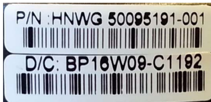
Figure 5-45-5: Part Number and Date Code (D/C) label on bottom of Terminal PCBA
