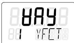
2. Use the
