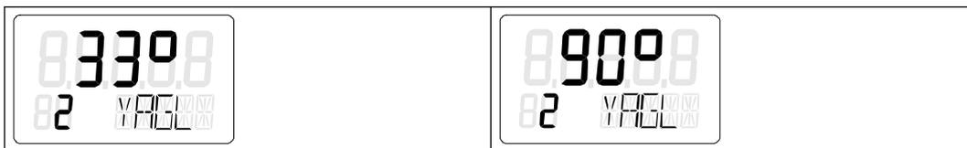
3. Check whether the value displayed of the "2.YAGL" parameter matches with the setting of the transmission ratio selector. If required, change the setting of the transmission ratio selector to 33° or 90°.
