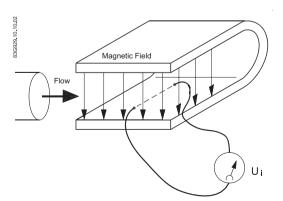
$U_i$  = When an electrical conductor of length L is moved at velocity v, perpendicular to the lines of flux through a magnetic field of strength B, the voltage  $U_i$  is induced at the ends of the conductor
