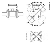
Figure 4-7 Horizontal installation, various terminal box positions
