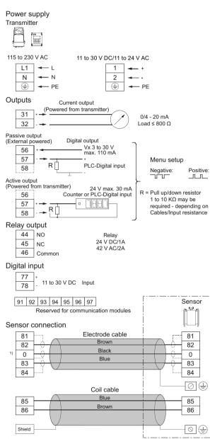
Note: Special cable with individual wire shields (shown as dotted lines) are only required when using empty pipe function or long cables.
