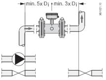
Figure 4-5 Inlet and outlet conditions
