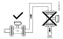
Figure 4-4 Correct installation at low point before outlet
