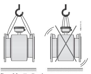
Figure 6-2 Handling of sensor
