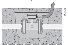
Figure 5-2 Direct burial of sensor
