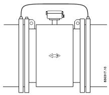
Figure 4-9 Cathodic protection
