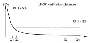
Figure 2-1 MI-001 verification tolerances
