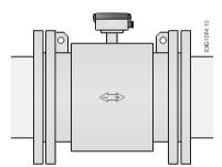
Figure 4-8 Potential equalization with earthing electrodes
