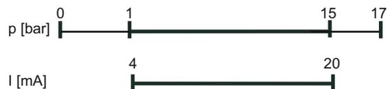
The measuring span is 14 bar.
