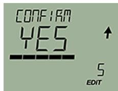
5. To validate the safety function, start the function test with "START". When you select "SKIP", you skip the function test and enable Functional Safety directly without validation of the safety function.
