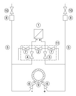
Pressure transmitter above the differential pressure transducer
