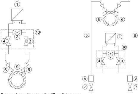
Pressure transmitter above the differential pressure transducer
