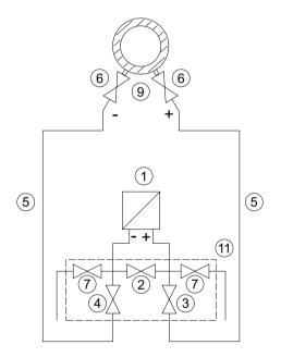
Pressure transmitter below the differential pressure transducer
