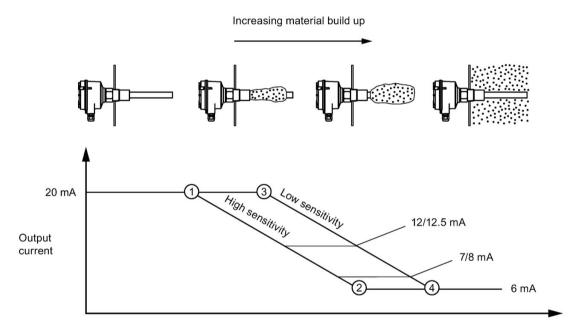
Vibration damping by material
