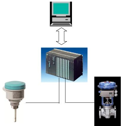
Figure 2-1: Example of a safety-instrumented system
