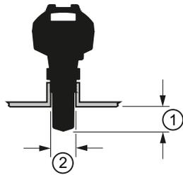
Stainless steel horn antenna
