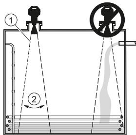
Flanged encapsulated antenna
