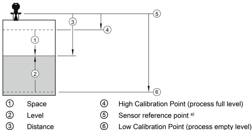
a) The point from which High and Low Calibration points are referenced: see **Dimension Drawings**.
