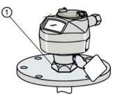
① Locking ring<sup>1)</sup> over threaded connection; secured by three 2 mm Allen set screws
