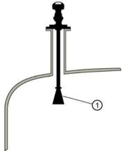
① If horn diameter is too large for the nozzle opening, insert it from inside the vessel.
