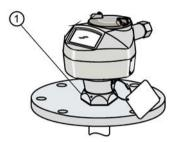
① Locking ring<sup>1)</sup> over threaded connection; secured by three 2 mm Allen set screws
