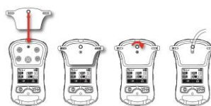
Install the calibration adapter on the QRAE 3 diffusion model
