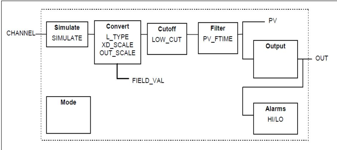
**Figure 7: Analog Input Block Schematic Diagram**
