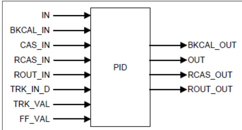
Figure 8: PID block
