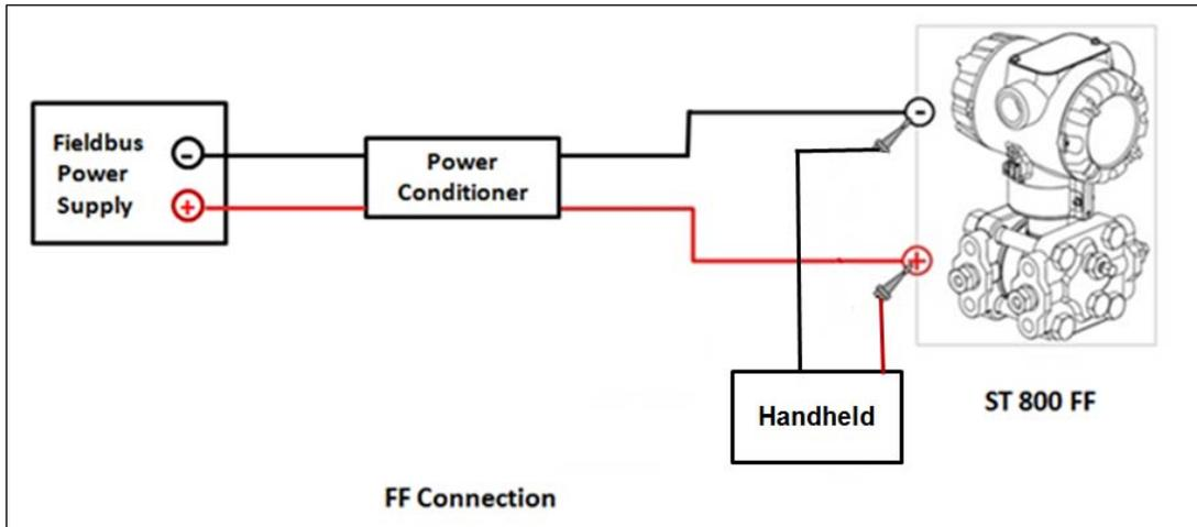
**Figure 18: Connecting the transmitter to the handheld**
