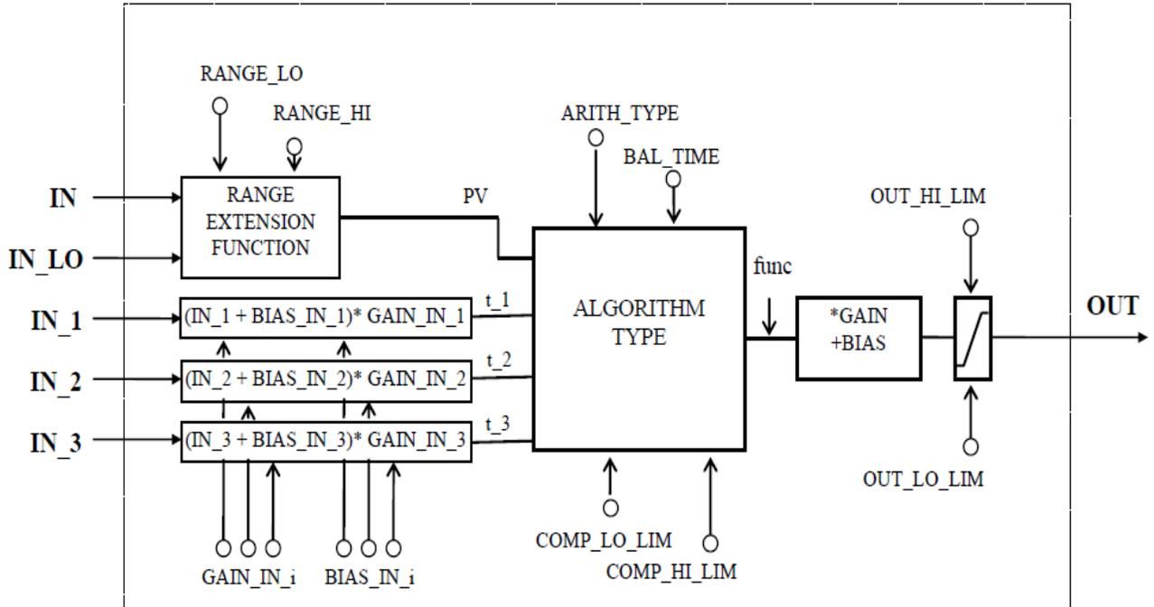
**Figure 15: Arithmetic schematic diagram**
