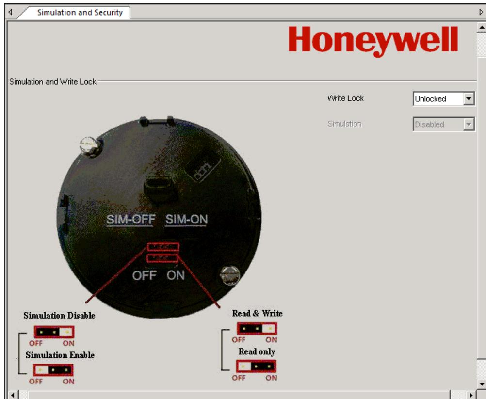
Figure 19: Simulation Jumper Location on Transducer Board
