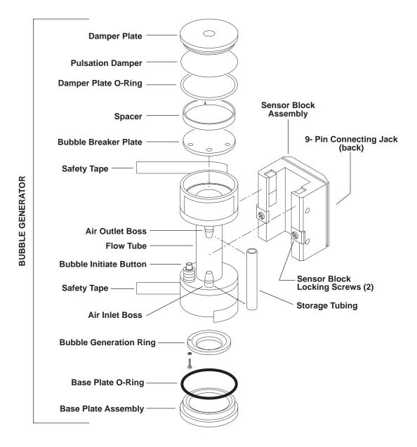
Figure 2.3 Wet Cell Assembly (Exploded View)
