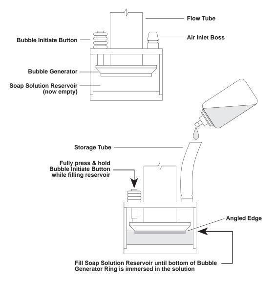
Figure 3.4 Adding Soap Solution (Wet Cell)
