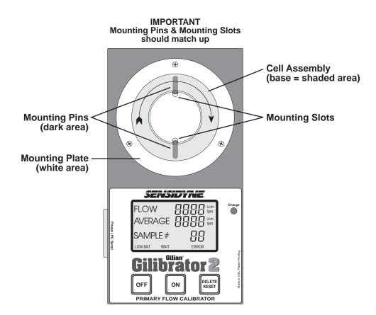
Figure 3.3 Cell Assembly Mounting (Top View)
