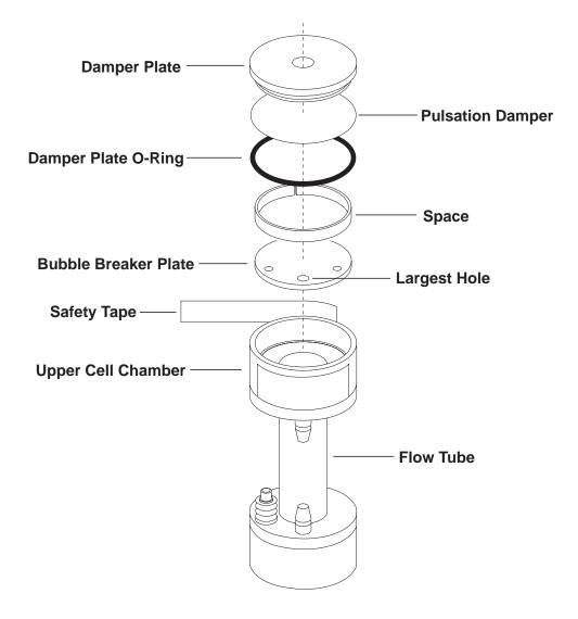
Figure 5.1 Wet Cell Assembly Maintenance
