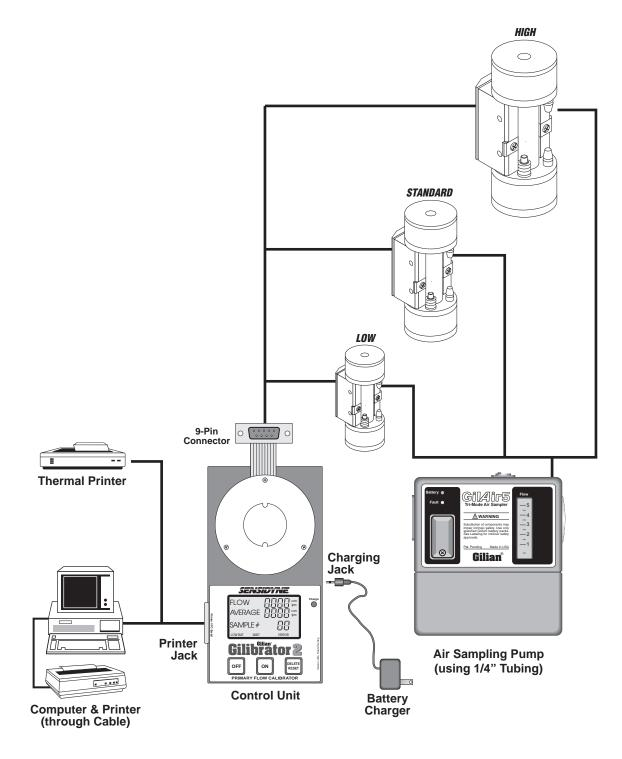
Figure 3.1 Gilibrator 2 System Setup
