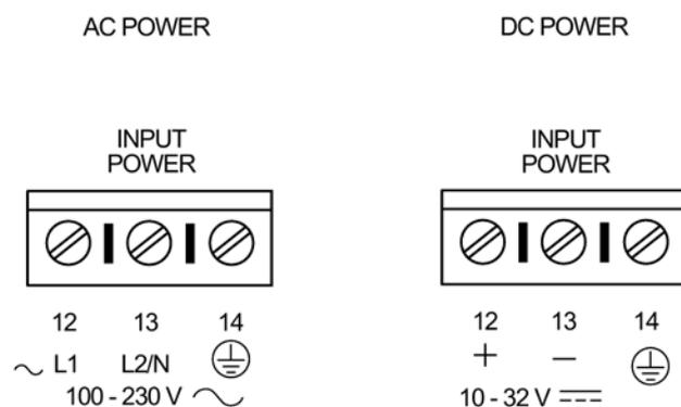
AC: 100-230 V AC 15%, 50/60 Hz, 36 VA (10W) DC: 10-32 V DC, 10W
