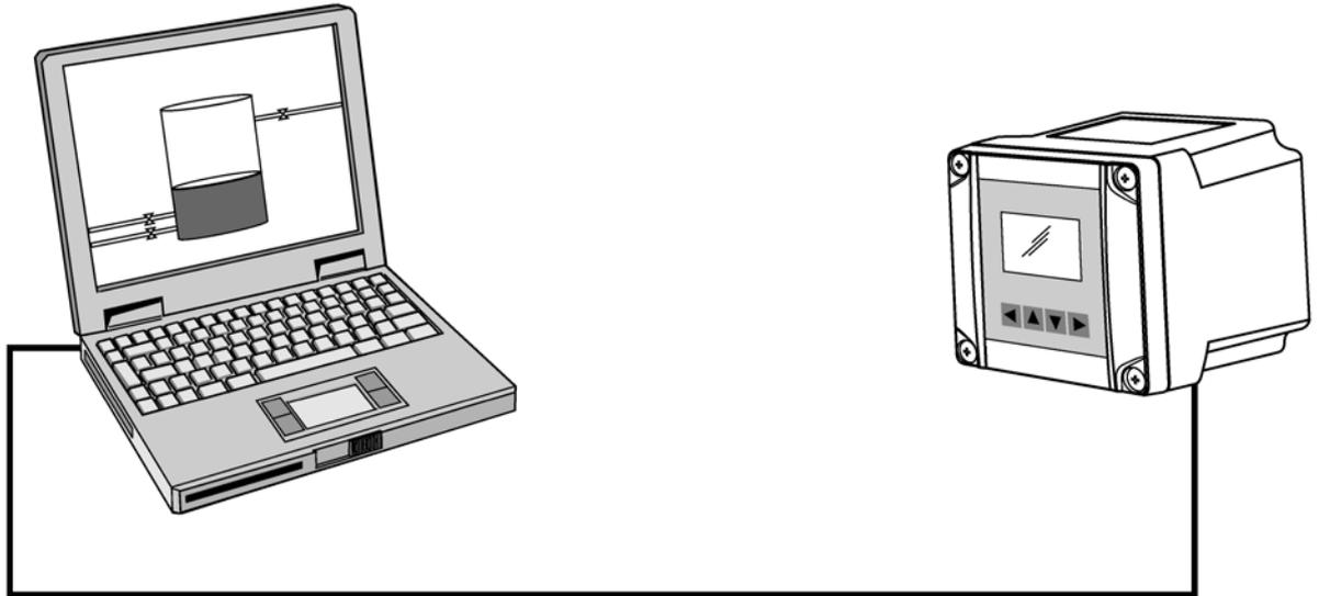
Figure 7-1 Communication via HART modem to SITRANS LUT400
