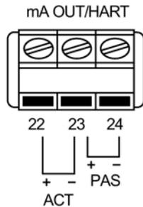
For ACTIVE HART connection (using LUT400 integral power supply), connect terminals 22 and 23.
