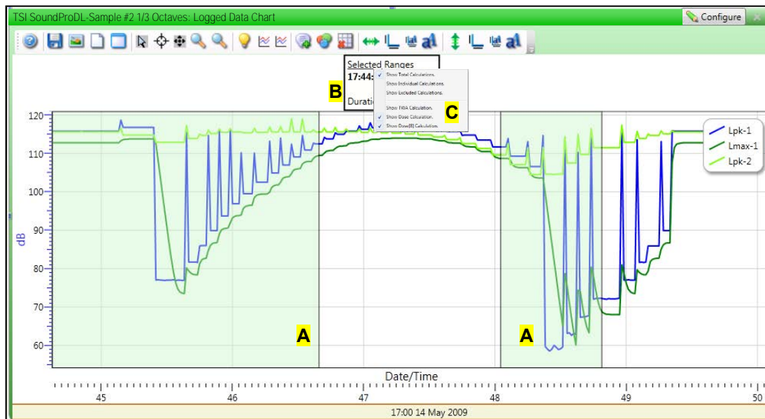
Figure 1-78: SoundPro meter and logged data chart with calculations
